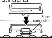
Select the dock insert for your Zune model from the table below and place insert in dock. Slide the Zune connector to left or right to match proper insert if necessary. Never dock a Zune without an insert in place.
